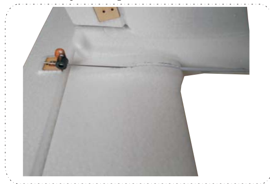
Control horn has been installed on the stabilizer
