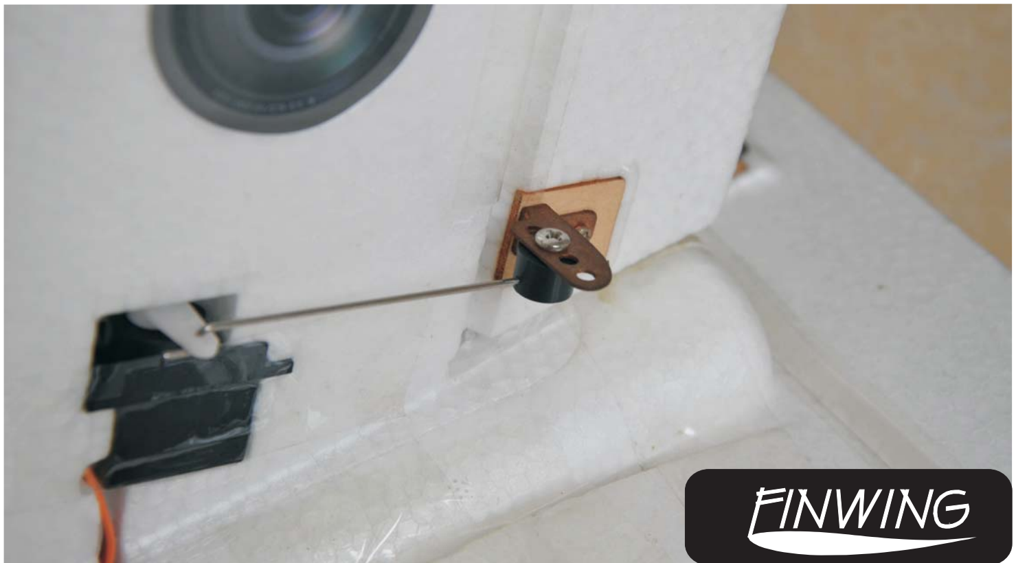
Vertical stabilizer (Rudder) _ Servo&Servo horn installation
