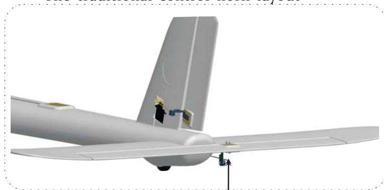
Control horn has been installed under the stabilizer
